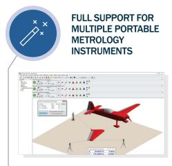
SA can simultaneously communicate with virtually any number and type of portable metrology instruments. This includes laser trackers, arms, laser radars, scanners, projectors, theodolites, total stations, and photogrammetric devices–all featuring a common interface for each instrument class.
